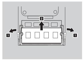
Align the notch of the DDR3 SDRAM with the protrusion of the socket and gently insert the DDR3 SDRAM into the socket at a 30-45° angle.
